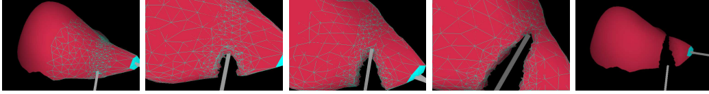
Figure 15: Result from [84] showing simulation of an invasive hepatic surgery simulator. They used a linear-elastic FE model that includes the notion of anisotropic deformation, or more specifically, the behaviour of a transversally isotropic material, where different stiffness properties of the material are defined in a given direction (2002).
